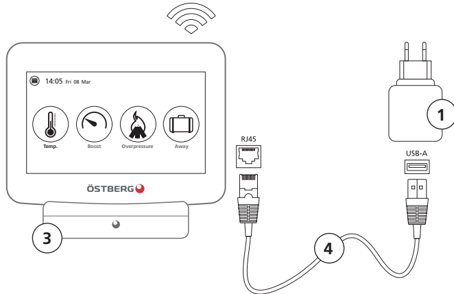
View C – Active dock holder – with USB-charger and RJ45/USB-A cable.
